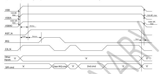
Figure 15: Power-up timing sequence
