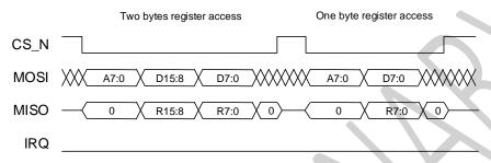
Figure 5: Principal SPI sequence for writing to a setup register
