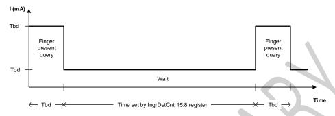
Figure 9: The fngrDetCntr register sets waiting time between finger present queries
