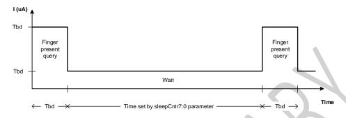
Figure 11: The sleepCntr parameter sets sleeping time between finger present queries in sleep mode.
