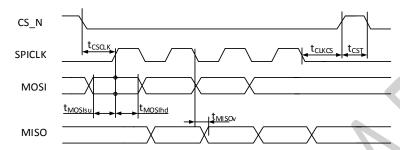
Figure 16: SPI timing
