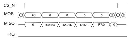
Figure 14: Principal SPI sequence for reading clock calibration result
