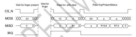
Figure 8: Principal SPI sequence for Wait for finger
