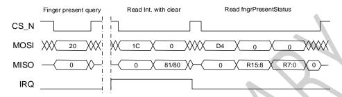
Figure 7: Principal SPI sequence for Finger Present Query
