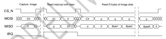
Figure 6: Principal SPI sequence for Image Capture
